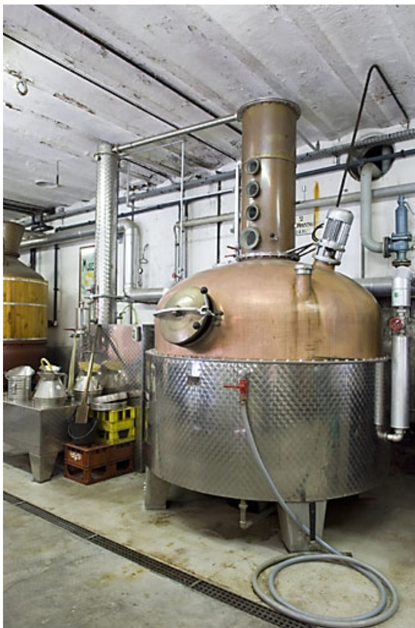
Atelier de distillation. Alambic Arnold Holstein.
