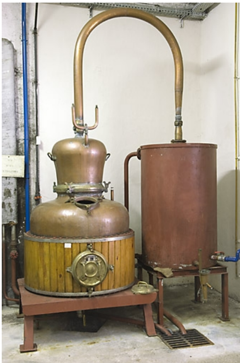
Atelier de distillation. Alambic Rump.
