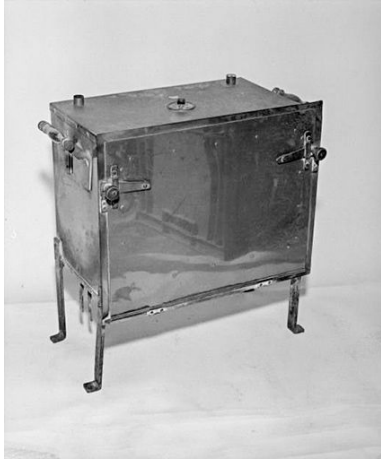
Autoclave. Phot. Jean-Luc Duthu IVR26_20067100343X
