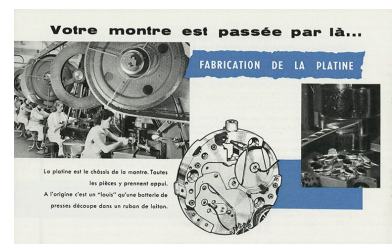
Fabrication de la platine, photogr., 1956. IVR43_20182500215NUC2A
