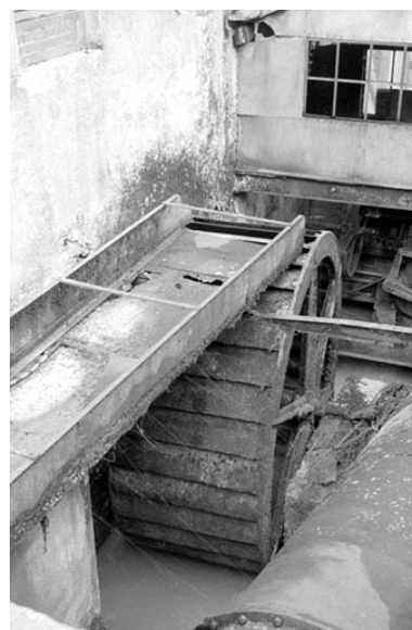
Roue hydraulique verticale. Phot. Laurent Poupard IVR43_19933900452Z
