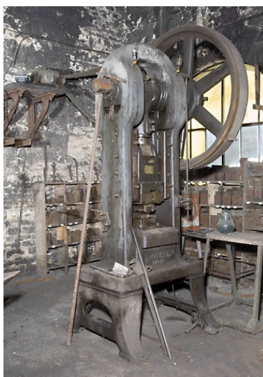
Atelier est. Presse à cisailler Bliss. Phot. Jérôme Mongreville IVR43_20087000815NUC2A
