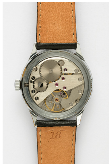
Mouvement Parrenin HP 60 G. Phot. Sonia Dourlot IVR43_20162500667NUC4A
